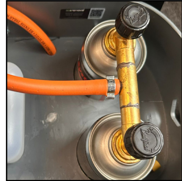
How to set the gas canisters up in the backpack
