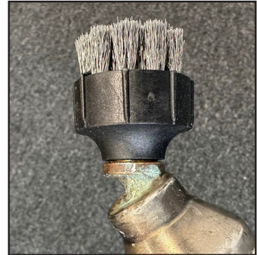
Attaching the brush to the lance
