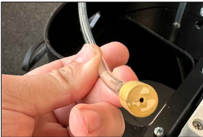
Brass coupler and fluid pipe which go inside the gum remover solution
